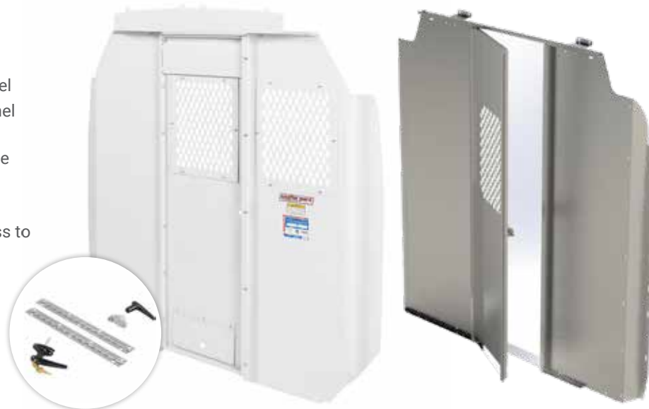
Steel Partition With Door
